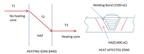
Moreover, when it be performed with local heat treatment because of any reason it can not be avoid heating gradient at heating boundary as we called "heating soak band" This heating soak band is similar to heat affect zone(HAZ) at welding, occurs 475 oC embrittlement. Therefore, the best way to stress releving method is to do furnance heat treatment. If heating and cooling temperature can not be strictly controlled. -The End--
