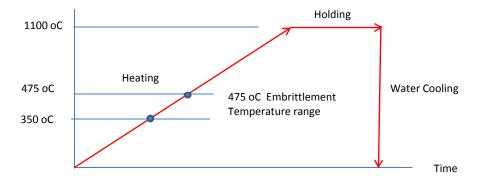
Therefore, all most of Cr-Mo Alloy material should be heat treated as method of water cooling in order to avoid 475 oC embrittlement after heating 1050 oC ~ 1100 oC there by, Cr can not be separated from Carbon grain.
